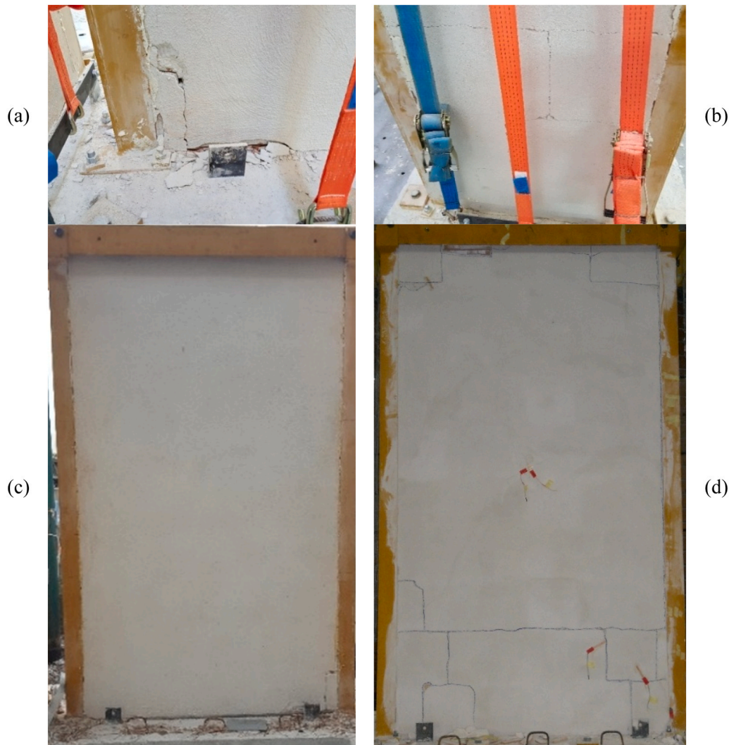
Fig. 7. Damage exhibited by the partition panels at the end of the incremental tests: (a) detail of the corner crushing for the wide partition panel (retrofitted (R) specimens), (b) detail of the wide sliding cracks in mortar in the joint between the bricks for the small partition panels (R specimens), and comparison between (c) R specimens and (d) non-retrofitted (NR) specimens [46].
